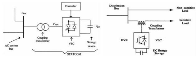
Fig 7. Schematic representation of the DSTATCOM
