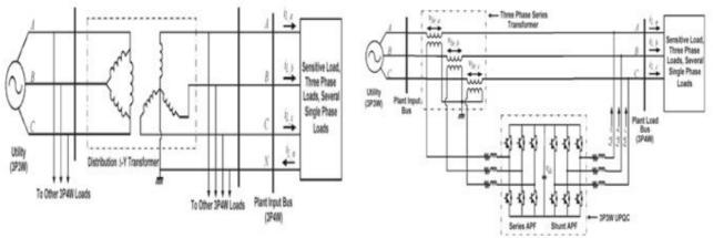
Fig. 11 3P4W distribution system: neutral provided from  $\Delta$ -Y transformer
