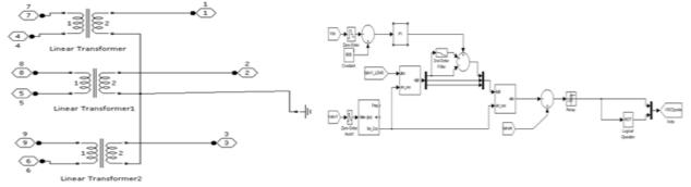
Fig. 16. Simulink diagram of three-phase series Transformer
