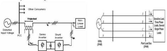
Fig 9 Basic Block Diagram of UPQC
